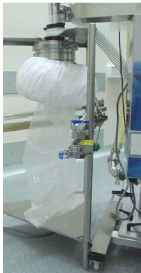
8. Continuous liner Tablet Collector
